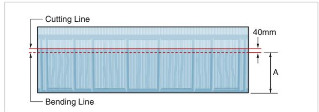
Note: It is essential to bend the Corona Shake before cutting to avoid Corona Shake distortion. Install the top course of Corona Shakes to the ridge board by nailing each Corona Shake through the up-stand to the batten in 4 places and nailing the bottom edge as previously described. Ensure that the top course of Corona Shake follows the same pitch as the other courses. Fig 3.6.3.
