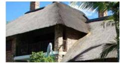
The traditional look of a thatch roof is its enduring quality. Though today, with many more electrical products in the home, smoking and cooking, the risk of fire is too great to contemplate it. A wet thatch roof after rainfall is also the ideal breeding ground for mosquitoes. Thatch also needs replacing periodically.
